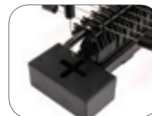
The damping unit with paddle and water bath can be used to generate running waves.
