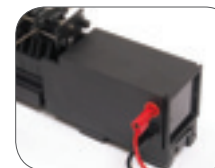
Motor powered eccentric driver can create traveling or standing waves.
