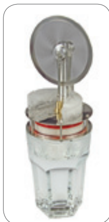
And is revived by ice on the top plate.
