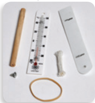
Assembled sling psychrometer includes wet and dry bulb thermometers.
