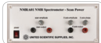
The scan control unit supplies an adjustable AC signal to the Helmholtz coils to scan the fixed magnetic field through a narrow range.
