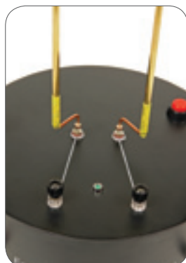
Pointed ends of the conductors fit into dimples in the top and bottom bearing contacts.
